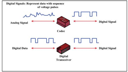
Analog and Digital Signaling of Analog and Digital Data
