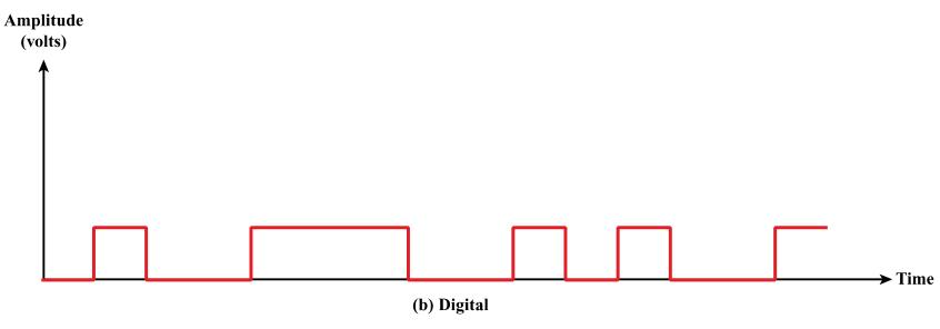
**Analog and Digital Waveforms**
