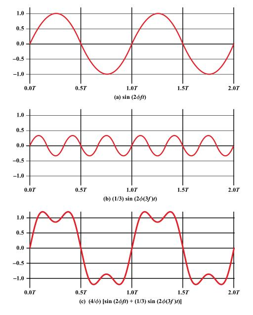
Addition of frequency Components(T = 1/f)
